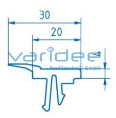
Reference: SEL8-2-4-Z Panel-clamping-strip 8 2-4 mm, grey (cut)
