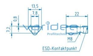
T-slot nut 8 St M8 with guiding ridge, ESD, galvanized
