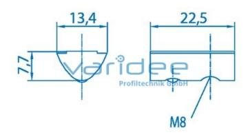
T-slot nut 8 St M8 with guiding ridge, galvanized
