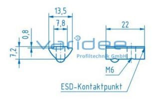
T-slot nut 8 St M6 with guiding ridge, ESD, galvanized
