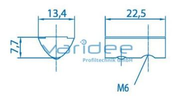
T-slot nut 8 St M6 with guiding ridge, galvanized
