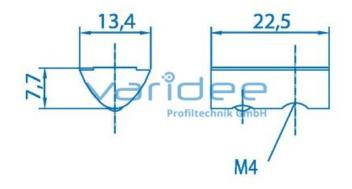
T-slot nut 8 St M4 with guiding ridge, galvanized
