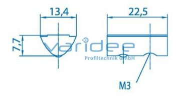
T-slot nut 8 St M3 with guiding ridge, galvanized
