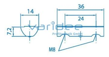
T-slot nut 8 St 2xM8-36 with guiding ridge, galvanized
