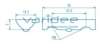
T-slot nut 8 St 2xM8-36, galvanized
