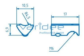
T-slot nut 6 St M6 with guiding ridge, galvanized
