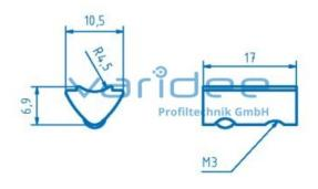
T-slot nut 6 St M3 with guiding ridge, galvanized
