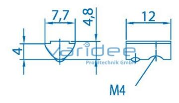
T-slot nut 5 St M4 with guiding ridge, galvanized
