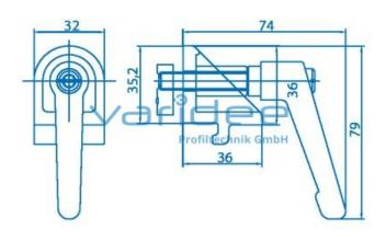
Angle clamp bracket 8 with clamp lever
