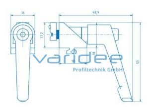
Angle clamp bracket 5 with clamp lever
