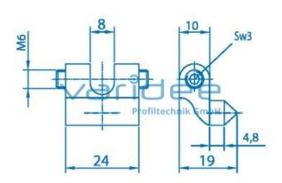
Clamping block 8 for corrugated mesh
