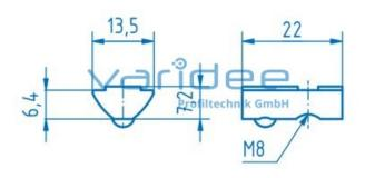
T-slot nut 8 St M8 with guiding ridge, with spring ball black, galvanized
