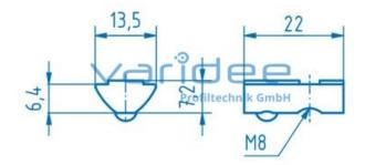
T-slot nut 8 St M8 with guiding ridge, stainless
