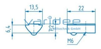
T-slot nut 8 St M6 with guiding ridge, stainless
