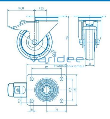
Castor D125 swivel, double-brake with mounting plate 140x110
