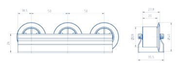
Roller Conveyor St ESD D30 with Flanged Wheel, black (cut)
