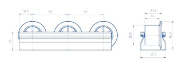
Roller Conveyor St D30 with Flanged Wheel, grey (cut)
