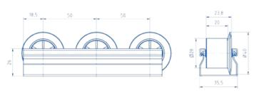
Roller Conveyor St ESD D30 with Flanged Wheel, black (2 meters)
