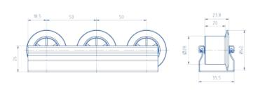
Roller Conveyor St D30 with Flanged Wheel, grey (2 meters)
