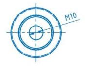
Threaded Insert, Profile Tube D30 M10 AI Reference: GWE-D30-AL-M10
