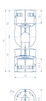
Ball Joint Butt Fastener D30 Al
