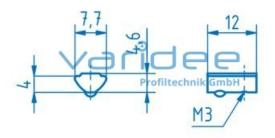
T-slot nut 5 St M3 with guiding ridge, galvanized
