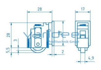
Roller set for Corner-Fastener 8 32x18
