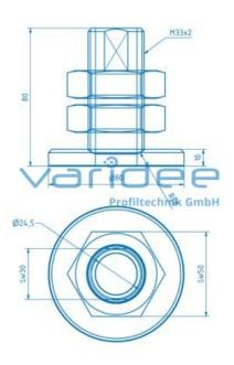
Levelling Feet D80, M33x80, galvanized
