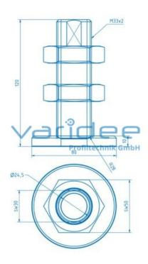
Levelling Feet D80, M33x120, galvanized Reference: NF-D80-120
