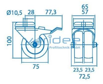
Double-castor D75 swivel, double-brake, galvanized
