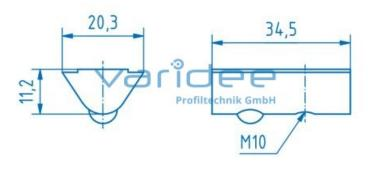
T-slot nut 12 St M10 with guiding ridge, galvanized
