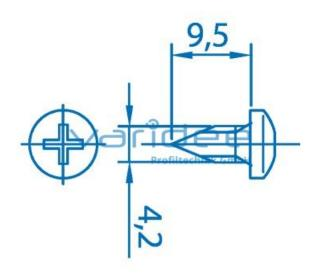
Tapping screw DIN 7981 St 4,2x9,5, galvanized
