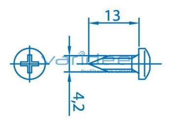
Tapping screw DIN 7981 St 4,2x13, galvanized
