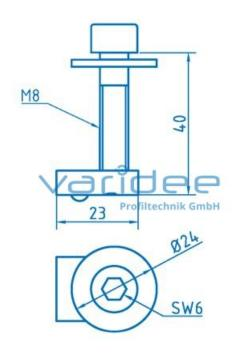
Fastening set 8 for castor swivel with lifting foot
