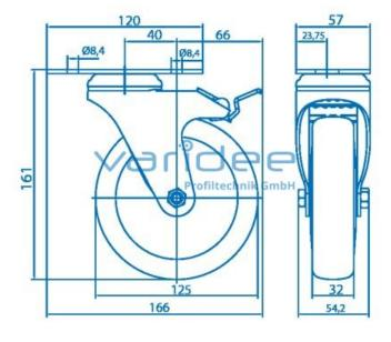
Castor D125 swivel, double-brake with mounting plate
