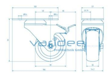
Castor D80 swivel, double-brake, mounting plate
