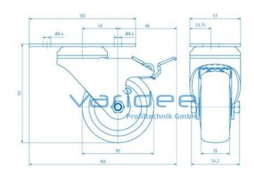
Castor D80 swivel, double-brake, mounting plate
