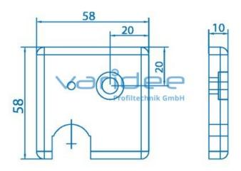
Wiper and lubricating system 8 D14, black Reference: ASS8-D14
